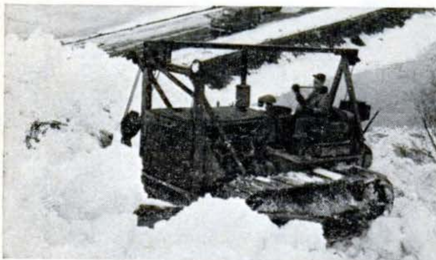
AVALANCHES that drag along trees and rocks are cleared away by bulldozers. Machine above works on a slide far up the mountain to prevent it from descending on the tracks.
